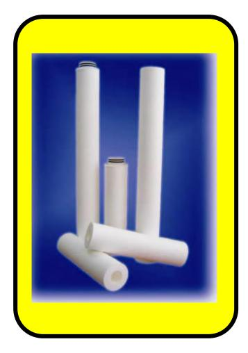
The melt blown Polyspun depth filter is an exceptional value for general applications where long life, high purity and low change-out frequency are required. Produced through a precise microfiber technology Polyspun is a 100% pure PP depth filter with exceptional dirt holding capacity. Polyspun true graded density filter matrix (lower density at the surface of the filter with progressively higher density towards the
