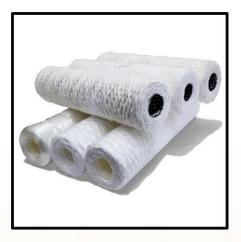
Maxi-Depth Precision Wound Depth Filter Cartridges are manufactured to give a considerable dirt holding capacity coupled with high flow rates and low pressure losses. Elements consist of a perforated support core of plastic or metal onto which yarn is wound at a pre-set rate, providing each rating of element with its own distinctive winding pattern and performance.
